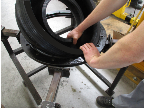
Figure 10: fix bellows to mounting ring
